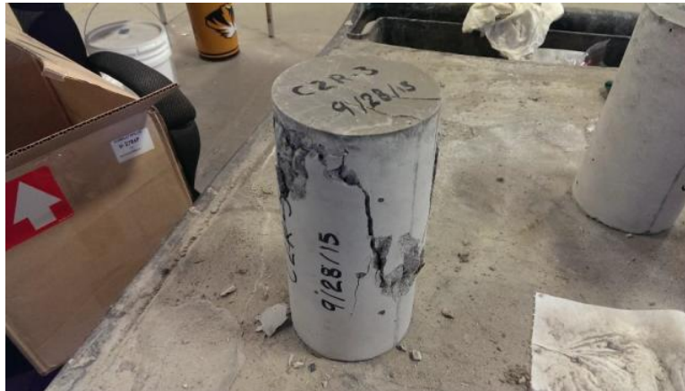
Figure 93 - Fractured cylinder after testing
