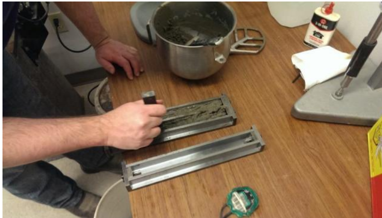
Figure 48 - Tamping mortar into molds
