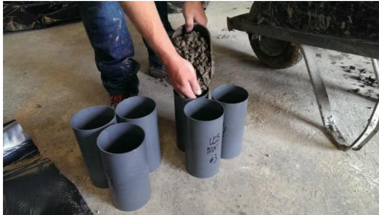
Figure 87 - Filling compression test cylinder molds
