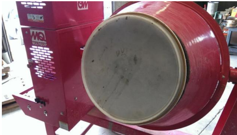
Figure 77 - Mixer is capped to prevent moisture loss during rest period
