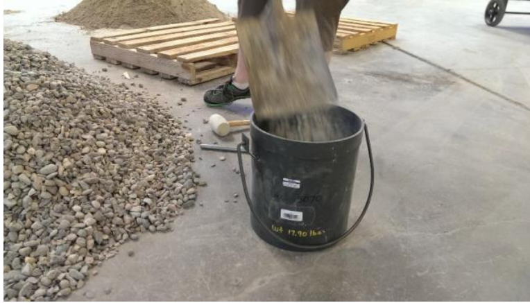
Figure 69 – Coarse aggregate is shoveled into the measure in three lifts.
