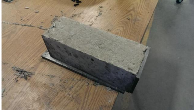
Figure 96 - Demolding a concrete prism.
