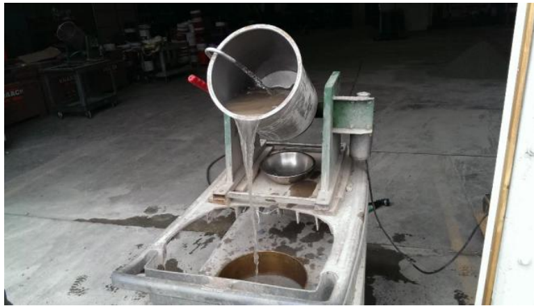
Figure 71- Washing aggregate in preparation for sieve analysis
