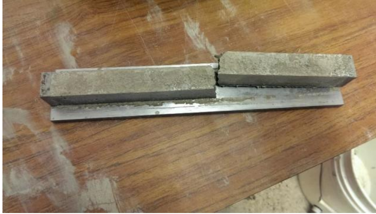
Figure 50 – This mortar bar broke during extraction
