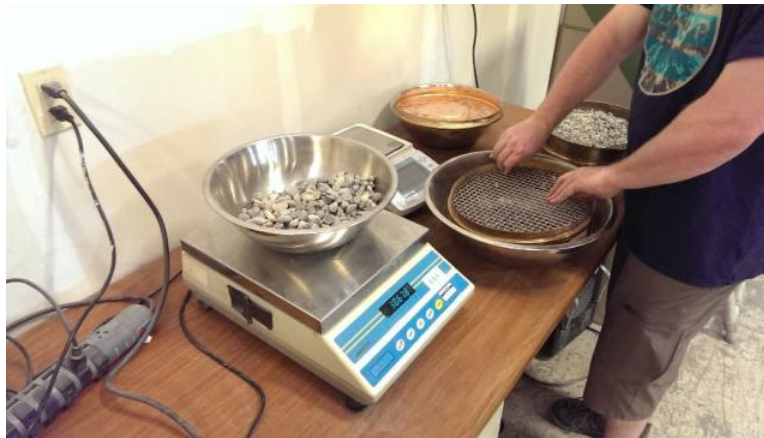
Figure 73 - Cleaning a screen during coarse aggregate sieve analysis
