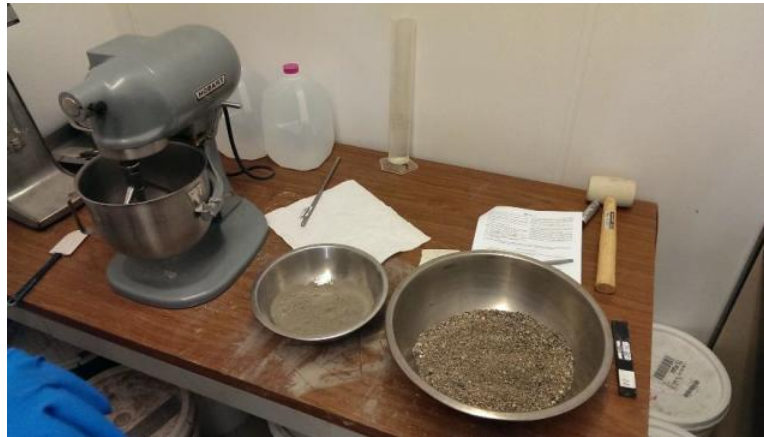
Figure 46 – Mixer with measured cement, water, and aggregate
