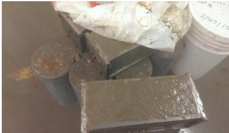
Figure 95 - 4 inch prisms are placed in fog room to cure 24 hours after casting.
