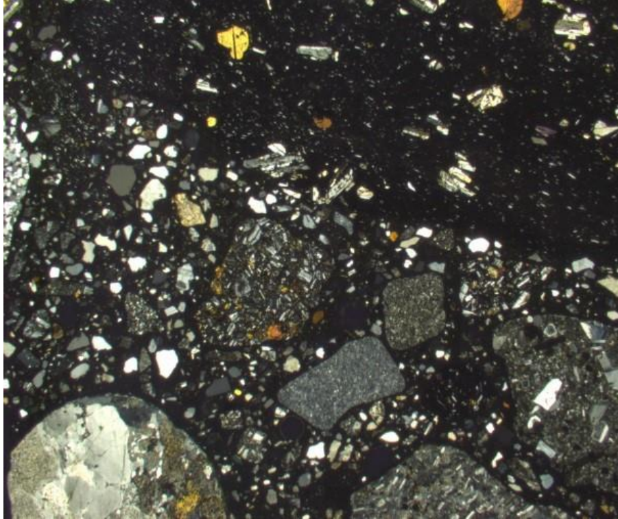
Figure 3: Concrete sample – the same area as in Figure 1 and 2. Cross polarized light. Magnification: x12.5
