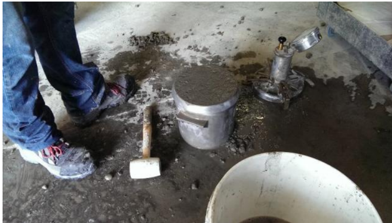
Figure 84 - After filling, the air meter bowl is struck off. Note the mallet used for tapping the bowl after each layer is rodded.
