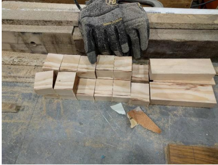
Figure 20 - Wooden blocks ready for installation in the jig.
