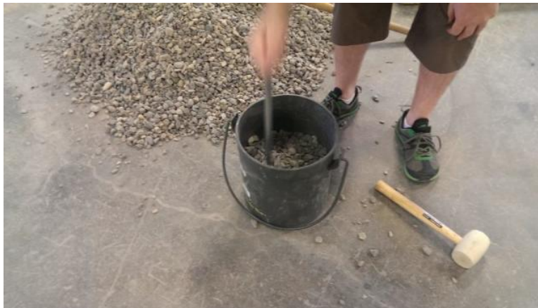
Figure 70 - Each lift is rodded 25 times.
