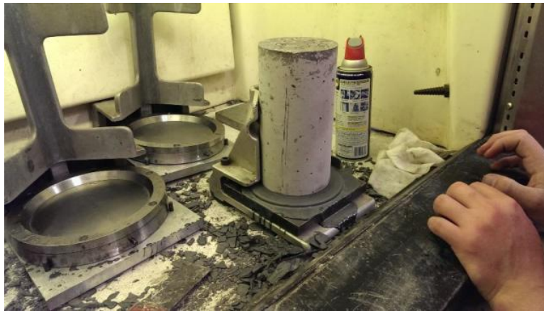
Figure 91 - Installing sulfur mortar end caps
