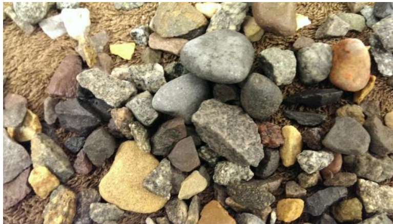
Figure 61 – Close up of coarse aggregate at saturated surface-dry condition
